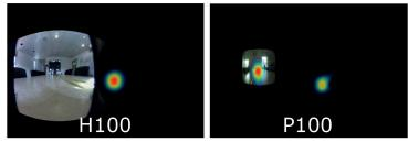
When imaging a weak source in the presence of a strong source, the H100 sees ony the strong source, but the P100 can see the weak source because of the P100's collimator.
